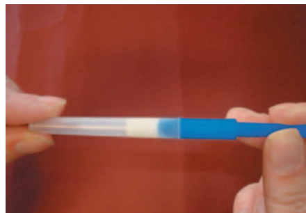
Keep pushing the stick into the sampling tube until it clicks.
