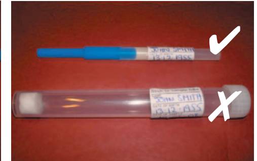
Label wraps around sampling tube NOT the transport tube.
